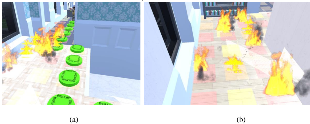
Figure 5. Illustration of the modeling for fire spreading, including the (a) paths divided into grid-based regions and (b) color indicators showing different risk levels for each region
