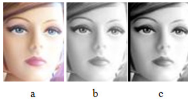
Figure 5: (a) Original dummy image (b) Gray scale dummy image (c) Dummy image after normalization: Illumination reduces
