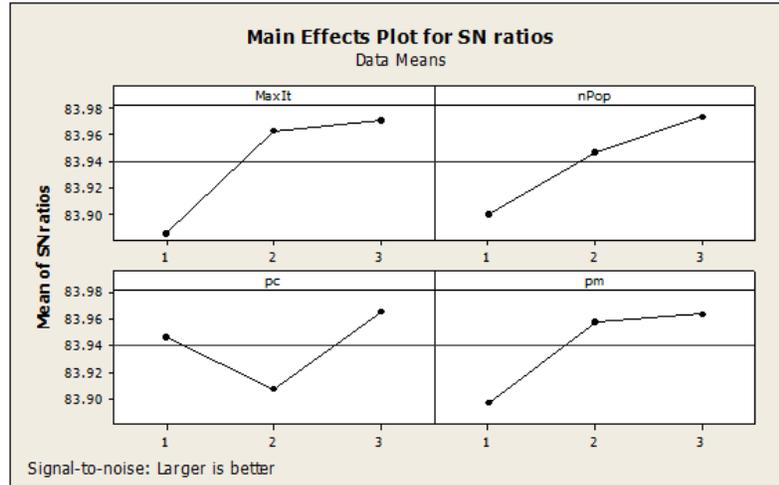
**Figure 3:** Mean S/N ratio for each level of the factors in the GA algorithm
