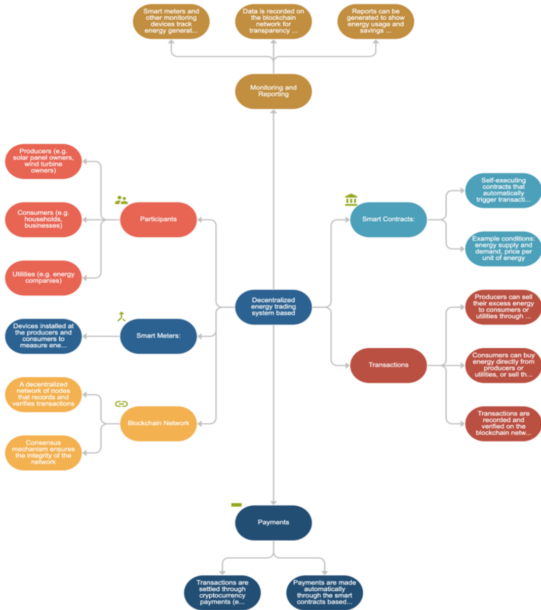
Figure 2 : Decentralized energy trading system based on blockchain
