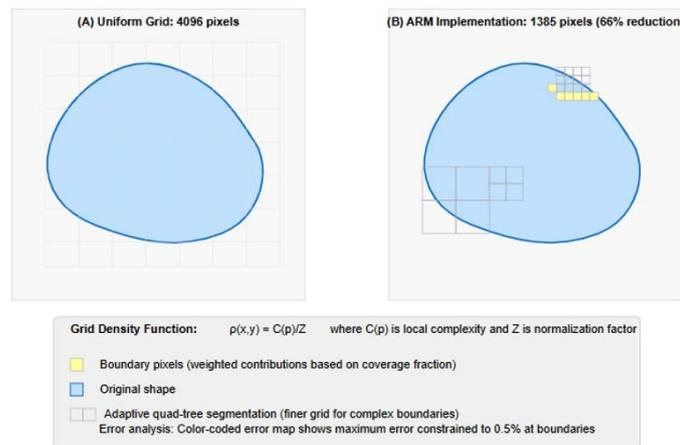
Figure 4: Illustration of ARM applied to an irregular shape, showing quad-tree segmentation with varying pixel density based on boundary complexity
