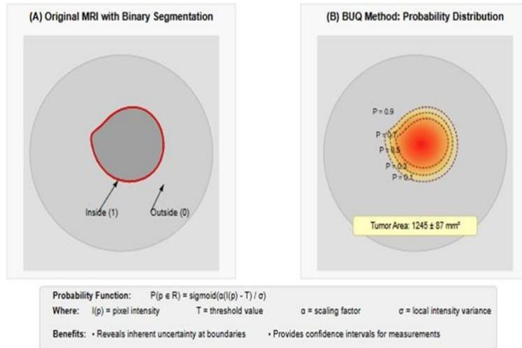
Figure 5: Boundary Uncertainty Quantification Applied to Medical Imaging
