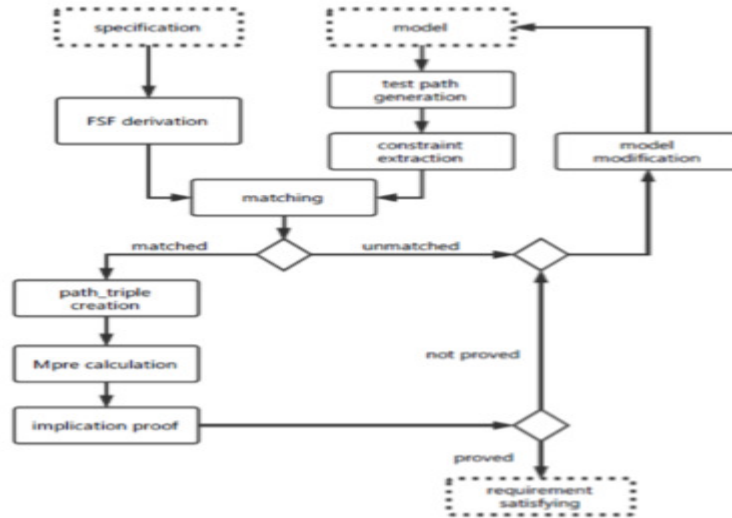
Figure 2. TBFV-M processing procedure
