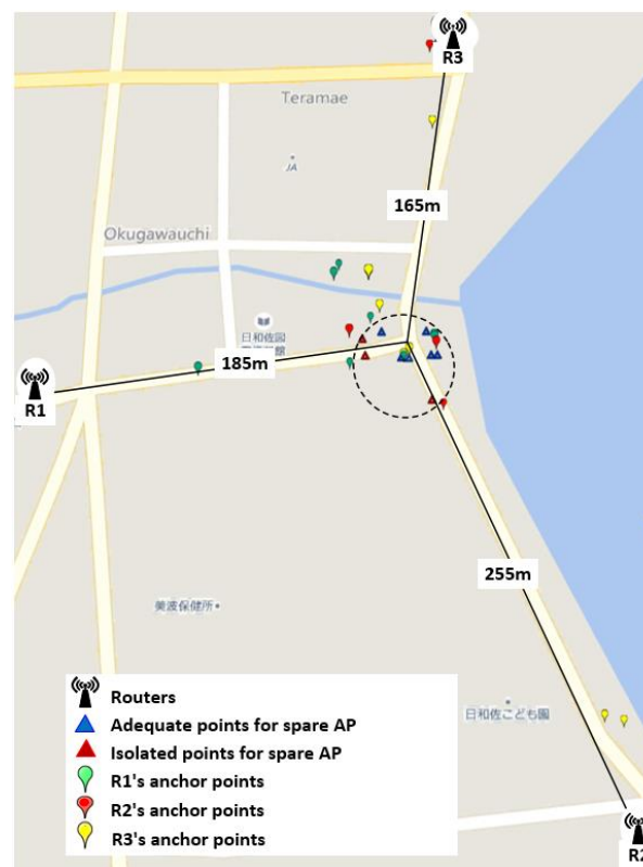
Figure 9. Router and Spare AP locations
