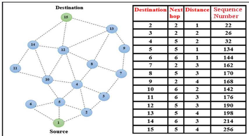
Figure 3. DSDV routing table for above nodes
