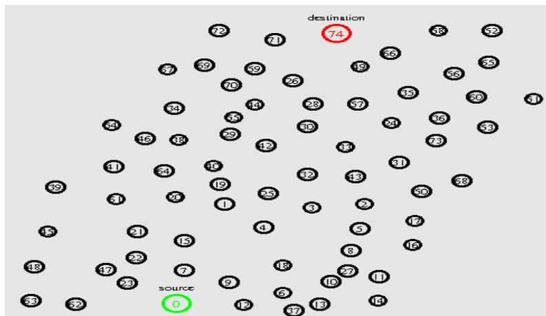
Figure 7. A WSN Topology with 75 sensor nodes used in simulation
