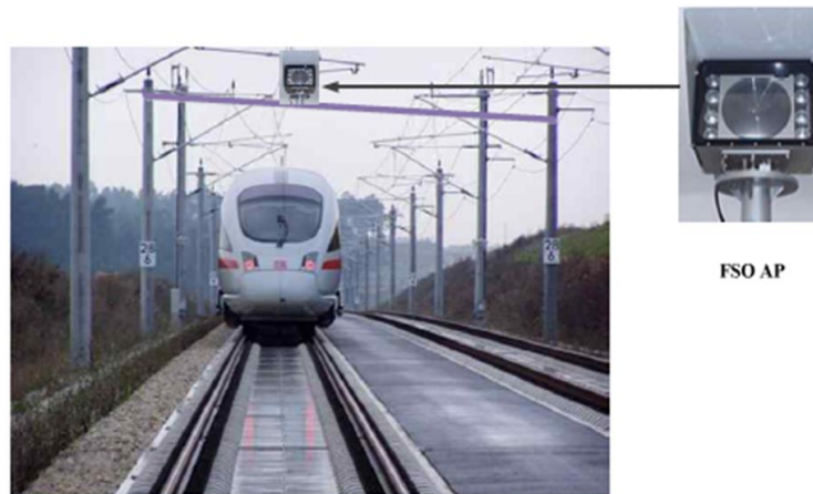
Figure 3: VLC outdoor application scenario where FSO communication is used for the users in train
