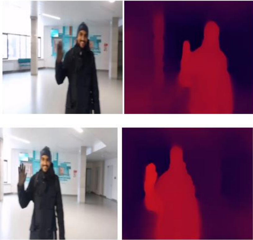
Figure 6 . A test video frames and their depth, the video has been taken by us using our hand-held phone (Huawei ) with motions , the depth estimations have a good quality and without any missing holes,however the motions in the video and movements of the camera.
