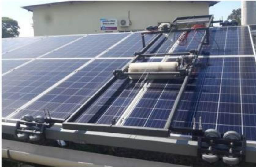
Figure 1: Cartesian robot developed
