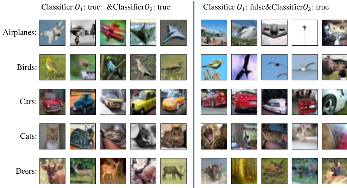
Figure 8. Sample results of output classifiers O_1 and O_2 for five CIFAR-10 classes. The left side shows easier instances where both classifiers made true classification, and the right side shows harder instances where only classifier O_2 made the true classification.
