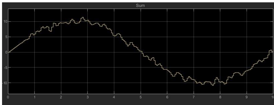
Fig 6(b) : Shows the Input Sine wave “Summed” with the Gaussian Random Noise (The Input Signal)
