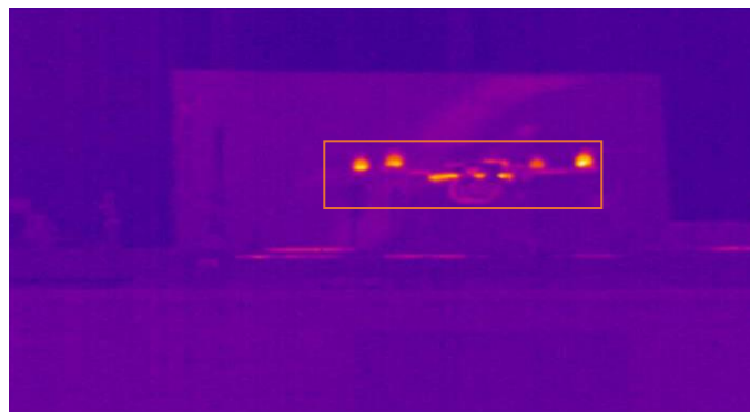
Figure 8. Quadcopter thermal image using Infrared technique [4].
