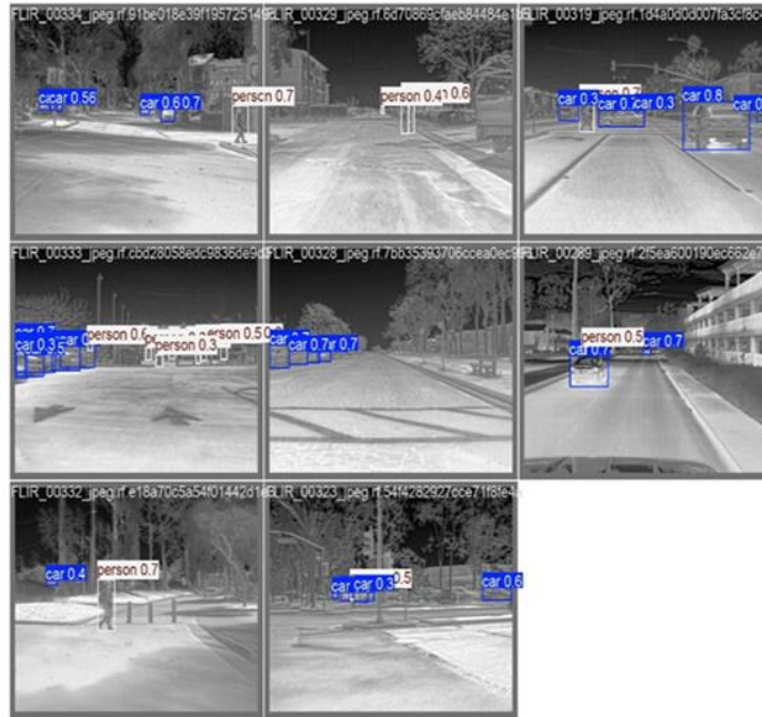
Figure 5. Object detection using proposed YOLOv8 on FLIR dataset
