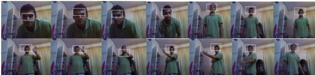
(a): Mean shift tracking results on the Face sequence. Frames left to right(upper) 1,19,50,164,203,251,304 and (bottom) 357,368,413,500,531,569,668 are displayed.
