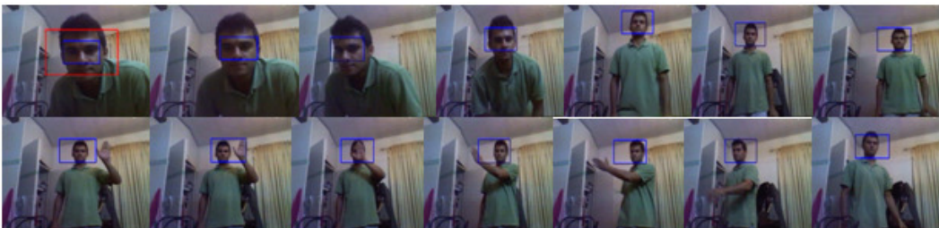
(b): CBWH tracking results on the Face sequence. Frames left to right(upper) 1,19,50,164,203,251,304 and (bottom) 357,368,413,500,531,569,668 are displayed.
