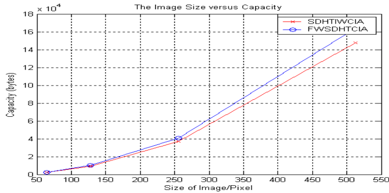
Figure 4. Comparisons Results of Size of Image/Pixel and Capacity (bits) among Varying Sizes of Embedded Lena Image with schemes SDHTIW CIA [7] and FWSDHTCIA
