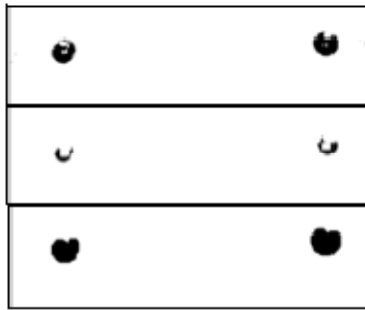
Figure 5. Pupils segmented (above), eroded (middle) and dilated (below).
