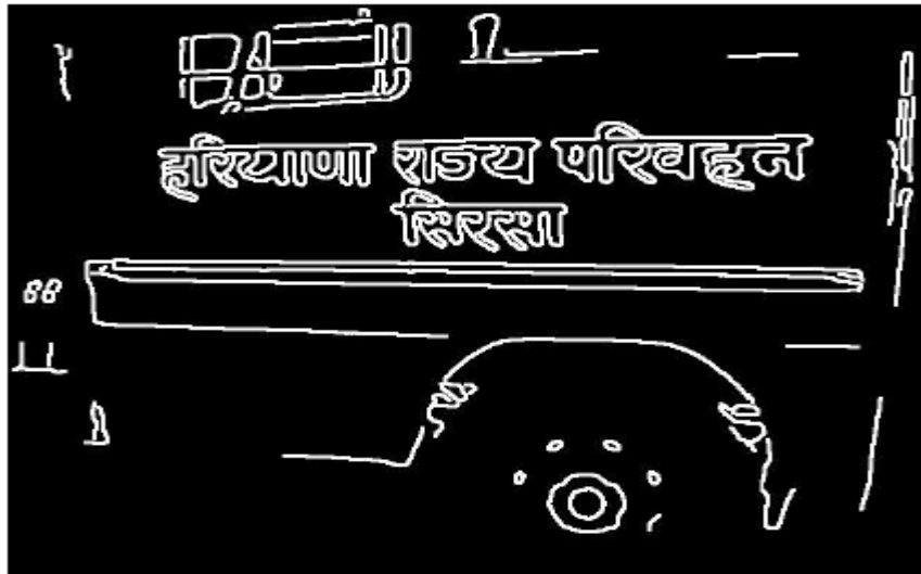
Figure 6 Edge Image after morphological dilation and eliminating border connected edges
