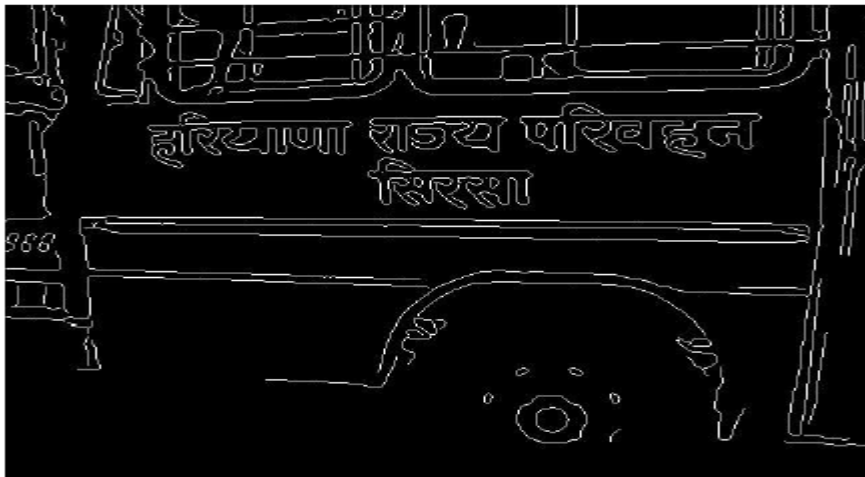
Figure 5 Edge Image formed by Canny Edge Detection
