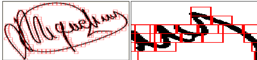
Figure 6. (a) Offline signatures image division. (b) A closer look at the windows for the signature part
