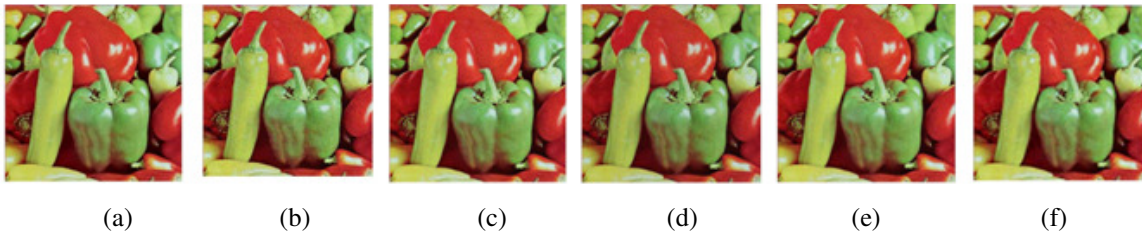
Fig 3 Results of Color image Peppers for visual perception. (a) Original Image, (b) Image with Gaussian noise, \sigma=15 . (c) Gaussian smoothing filter, (d) AFD filter, (e) AFI filter, (f) Proposed filtering method.
