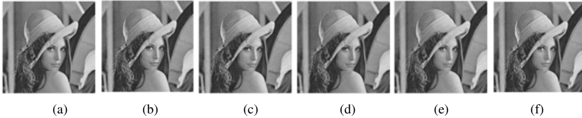
Fig 2 Results of Grayscale image Lena for visual perception (a) Original Image, (b) Image with Gaussian noise, \sigma=15 , (c) Gaussian smoothing filter, (d) AFD filter (e) AFI filter (f) Proposed filtering method.
