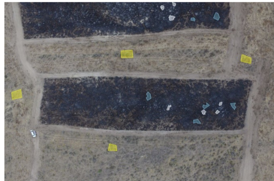
Figure 2. Training regions from a prescribed burn image. Training regions were used for calculating information gain to identify optimal texture measures. White regions are white ash, blue regions are black ash and yellow regions are unburned vegetation.
