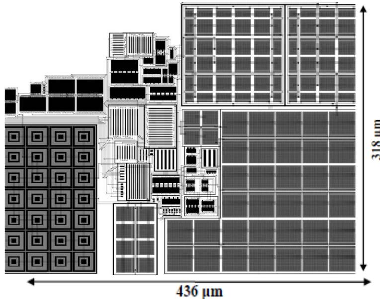
Figure 9: Layout of the proposed bandgap reference
