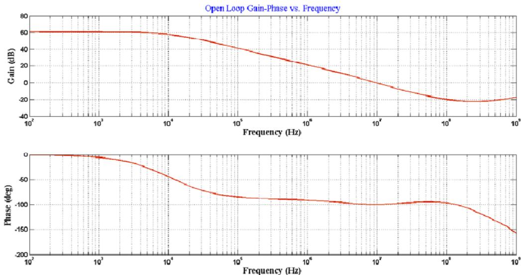
Figure 4: Gain and phase plot of the opamp
