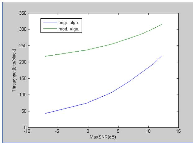
Figure.5.. Throughput vs maximum transmit power for second set of input for MRC scheme.
