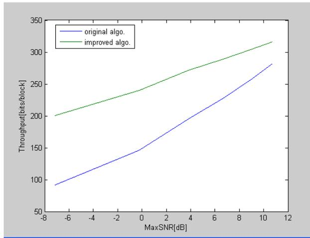
Figure.4. Throughput vs maximum transmit power for one set of input for MRC scheme.
