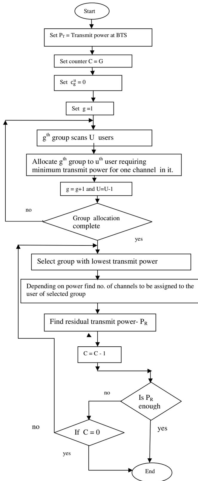
Figure. 2 Flowchart for original algorithm
