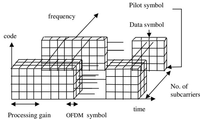
Figure.1 Frame format of sub carrier selecting MC-CDMA system .
