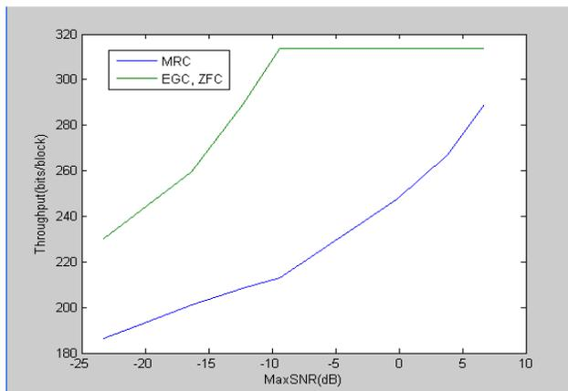
Figure.7. Throughput vs maximum transmit power power using modified algorithm.
