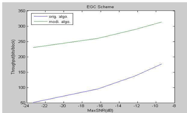
Figure.6.. Throughput vs maximum transmit power for EGC and ZFC scheme.
