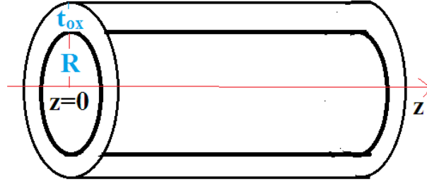
Figure 1 Cylindrical surrounding gate MOSFET (here only channel region with gate oxide is shown for simplicity)
