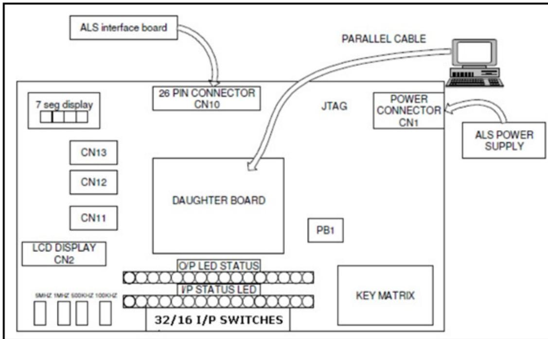
Fig.3 Connection diagram of Base-Board
