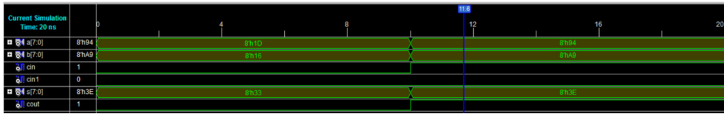
Figure 3. Simulation result of two 8-bit addition using CIA_RCA
