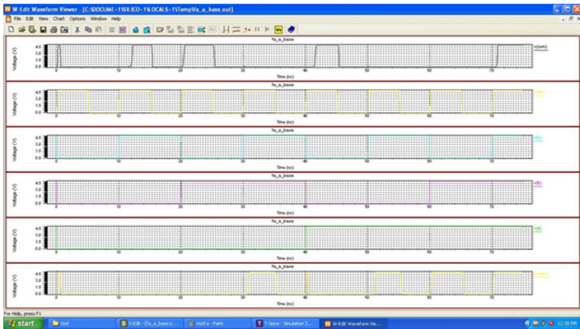
Fig.5. Simulation waveforms of adder 1
