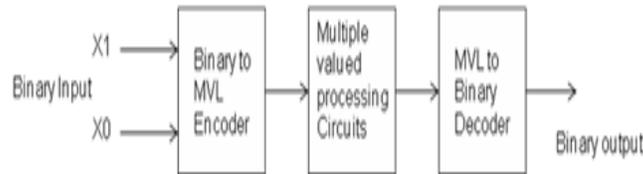
Figure 2. MVL circuit with multi valued processing
