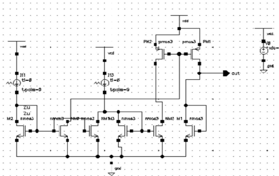
Figure 9. Schematic of Max Gate Circuit
