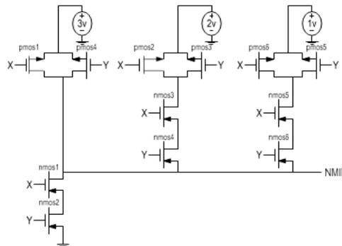
Figure 5. Schematic of Quaternary NMIN gate [5]
