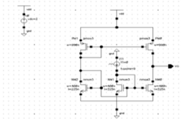
Figure 10. Schematic of comparator Circuit
