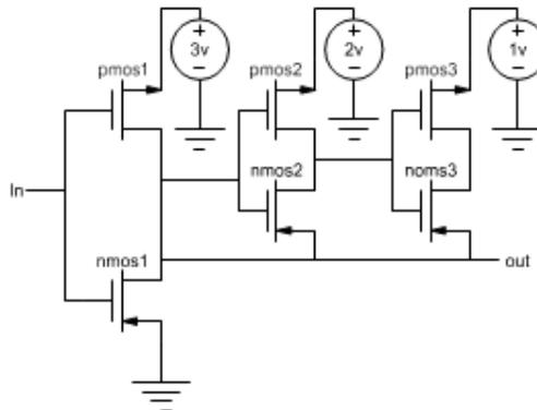
Figure 4 . Design of quaternary inverter [5]
