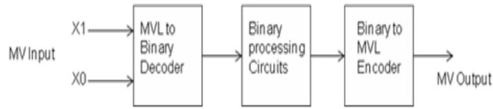
Figure 1. MVL circuit with binary processing
