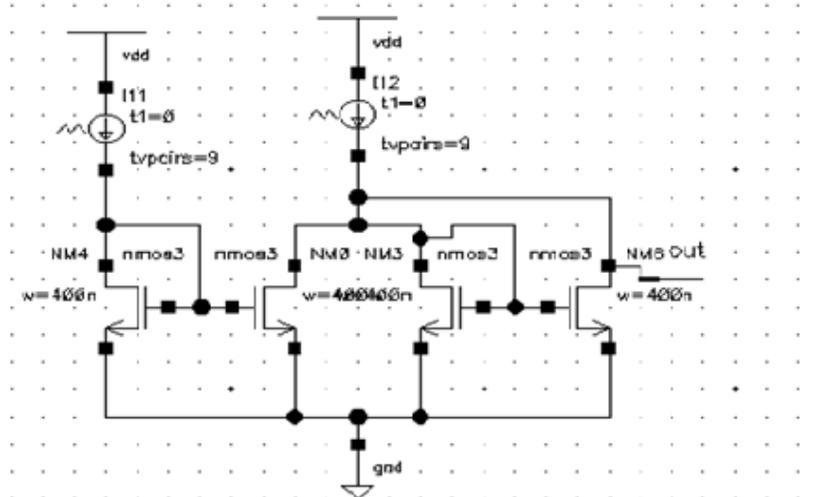
Figure 8. Schematic of Min Gate Circuit
