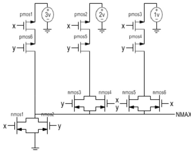
Figure 6. Schematic of Quaternary NMAX gate
