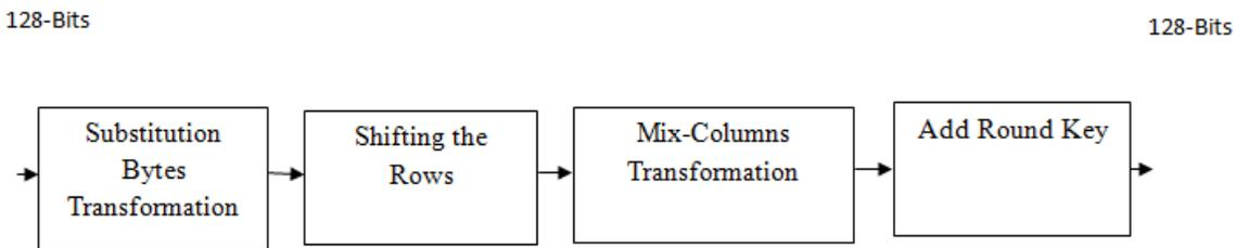
Figure 1: Flow Diagram for Advanced Encryption Standard Architecture
