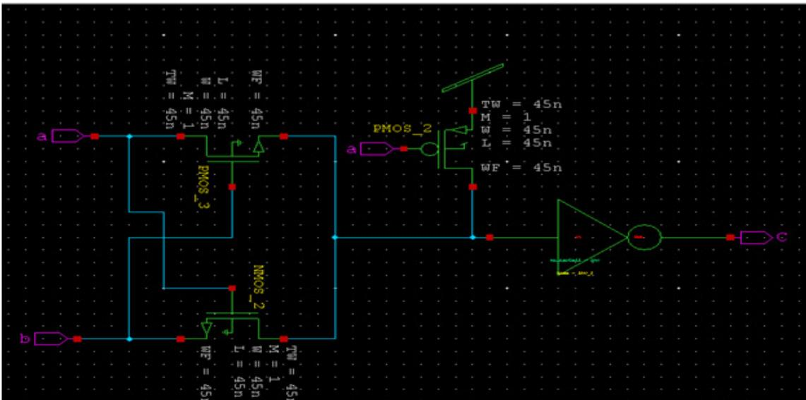
Figure 6: Proposed Nano-Wire based XOR gate
