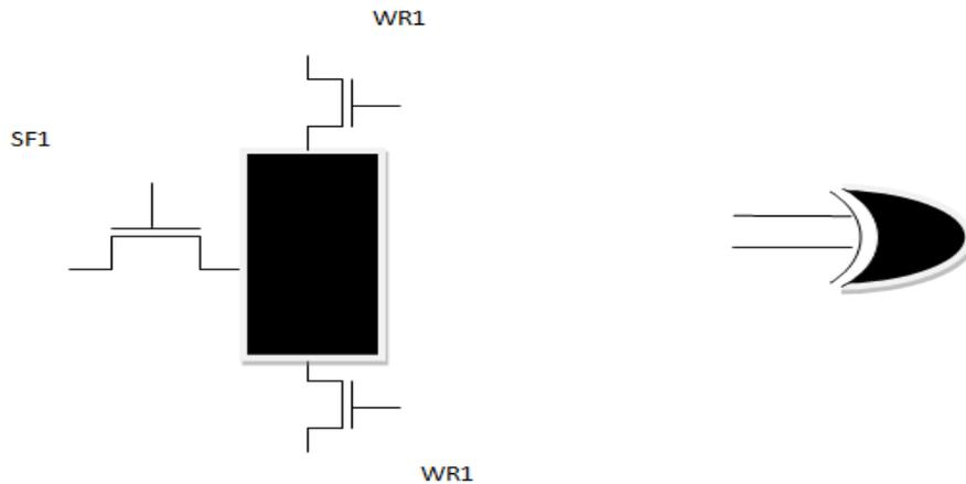
Figure 3: Nano wire based XOR Gate and Symbolic View of the XOR Gate
